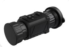
HikMicro THUNDER Pro TQ50C Thermal Monocular has  $640 \times 512$  thermal detector and  $1024 \times 768$  OLED monitor, which provides clear image under harsh environment conditions like darkness, fog, smoke, dust, rain, snow, wood, camouflage, etc. The scope is mainly applied to scenarios such as hunting.
